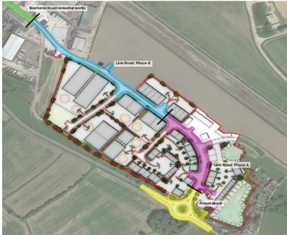
Figure 5.a: Sketch of Ashbourne Airfield Roundabout & Link Road showing constituent elements as costed
