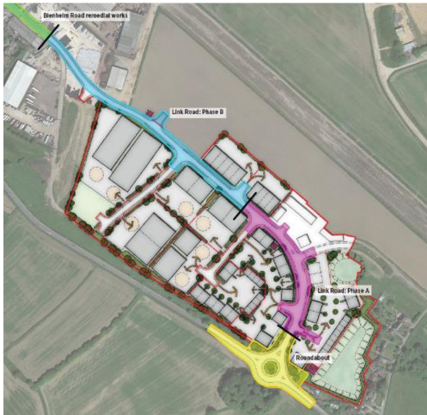
Figure 1.d: Sketch of Ashbourne Airfield Roundabout & Link Road showing constituent elements
